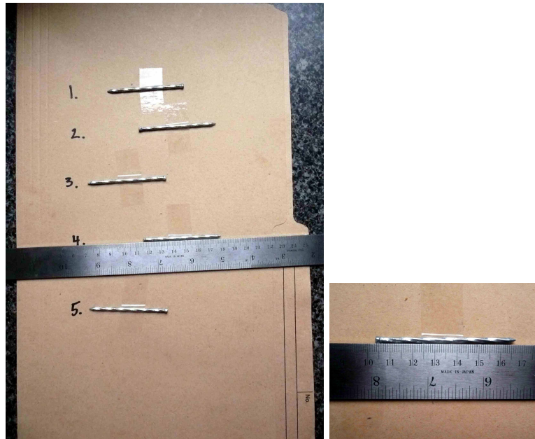
FIG. 1 – Left : notice the irregular placement of the nails on the cardboard ; notice also that there is enough space between nails to insert the ruler easily. Right : notice that the ruler was randomly placed near the nail.
