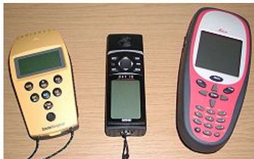
Fig. 4 – Left: pocket GPS receivers ; right : vessel GPS serving to establish and control trajectories.
